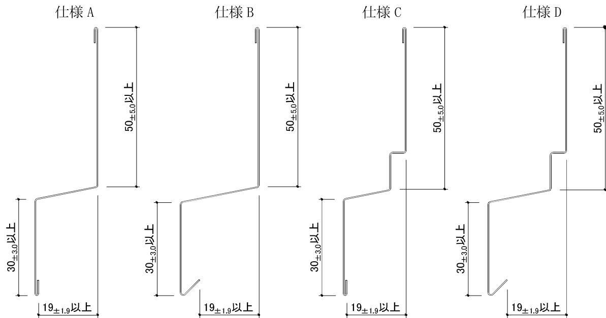
外装材接合部材（端面カバー）の代表例
